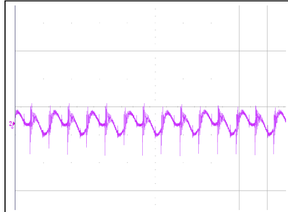
Figure 2: AGF600-48S28-6L Ripple and Noise Measurement Ch 2: Vo (5us/div, 50mV/div)
