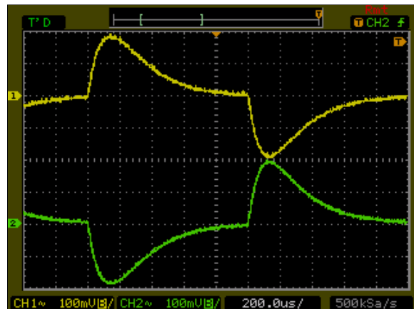
Figure 139: ATA00CC36-L Transient Response Vin = 48Vdc, Load: Io = 100% to 75% load change, Ta=25 °C Ch 1: V1 Ch 2: V2
