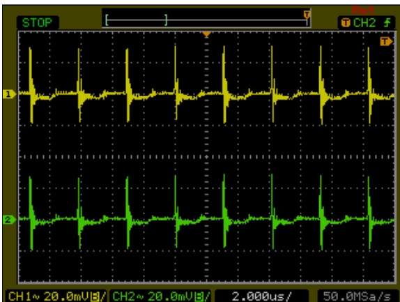
Figure 120: ATA00AA36-L Ripple and Noise Measurement Vin = 48Vdc, Load: Io = ±0.3A, Ta = 25 °C Ch 1: V1 Ch 2: V2
