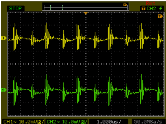
Figure 129: ATA00BB36-L Ripple and Noise Measurement Vin = 48Vdc, Load: Io = ±0.125A, Ta = 25 °C Ch 1: V1 Ch 2: V2
