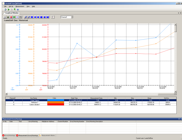
Fig. 1: The graphical window shows up to seven graphs. The user selects the data plotted, the scaling, and the style and color of the lines and background to build the graphical window.
