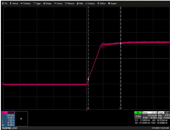
Figure 10: LCM4000HV-T Output Startup Characteristic Vin = 311Vac Load: R = 15.62 ohm Ch 2: Io
