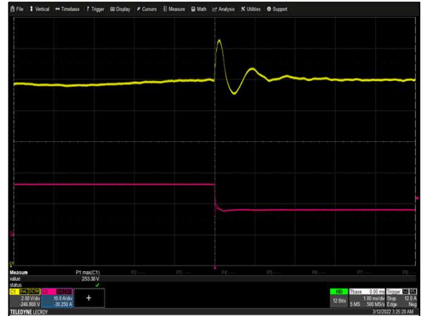
Figure 8: LCM4000HV-T Transient Response - Vo Deviation 100% to 50% load change, 1A/uS slew rate Vin = 380Vac Ch 1: Vo Ch 2: Io
