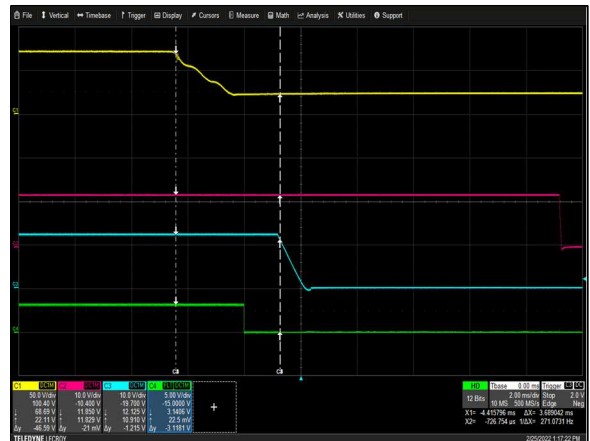
Figure 4: CSU1300ADC-3-100 Hold-Up Time Vin = -72Vdc Load: I O = 106.5A I SB = 3.5A Ch 1: V IN Ch 2: V SB Ch 3: V O Ch 4: PWOK
