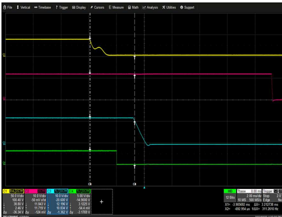
Figure 3: CSU1300ADC-3-100 Hold-Up Time Vin = -40Vdc Load: I O = 106.5A I SB = 3.5A Ch 1: V IN Ch 2: V SB Ch 3: V O Ch 4: PWOK
