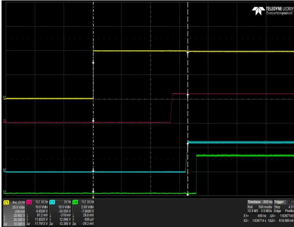
Figure 1: CSU1300ADC-3-100 Turn-On Delay via DC input Vin = -40Vdc Load: I O = 106.5A I SB = 3.5A Ch 1: V IN Ch 2: V SB Ch 3: V O Ch 4: PWOK
