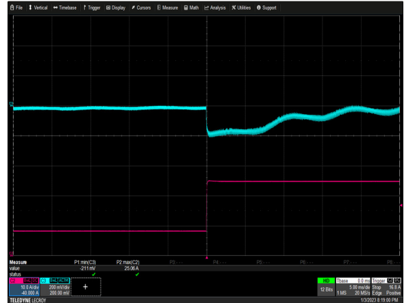
Figure 19: NGB800S24K Transient Response - Vo Deviation Vin = 115Vac Load: Io = 25% to 75%, 0.2A/ \mu s slew rate Ch 2: Io Ch 3: Vo
