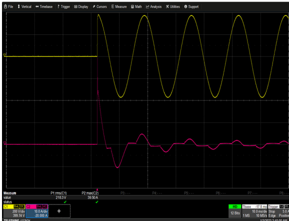
Figure 14: NGB800S24K Inrush Current Vin = 264Vac Load: Io = 0A, Turn on at 90 deg Ch 1: V_{IN} Ch 2: I_{IN}
