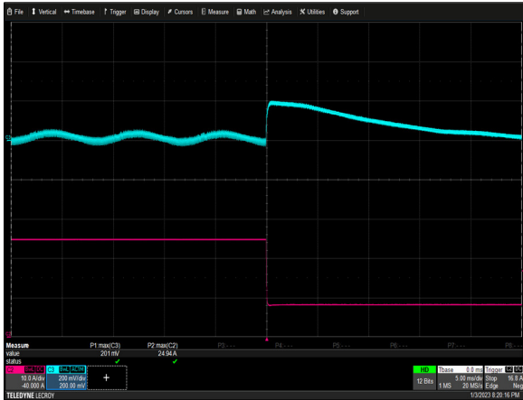
Figure 18: NGB800S24K Transient Response - Vo Deviation Vin = 115Vac Load: Io = 75% to 25%, 0.2A/ \mu s slew rate Ch 2: Io Ch 3: Vo
