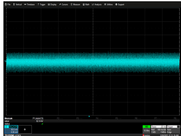
Figure 6: NGB800S12K Ripple and Noise Measurement Vin = 115Vac Load: Io = 57.5A Ch 3: Vo
