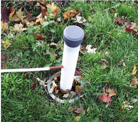
Fig.1 The soil gas probe with the sampling tube connected
