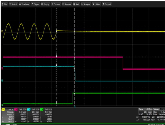
Figure 21: μMP10T-S2Q-S2Q-S2Q-S2Q-S2Q-S2Q-90-A Hold-up Time via AC mains Vin = 90Vac/63Hz Load: I O = 41.66A I SB = 2A Ch 1: AC Mains Ch 2: V SB Ch 3: V O Ch 4: Global DCOK
