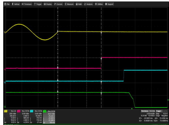
Figure 28: μMP10T-S2Q-S2Q-S2Q-S2Q-S2Q-90-A AC OK Delay - Turn off V_{in} = 90Vac Load: I_o = 41.66A Ch 1: V_{IN} Ch2: Input AC OK Ch3: Global DC OK Ch4: V_o
