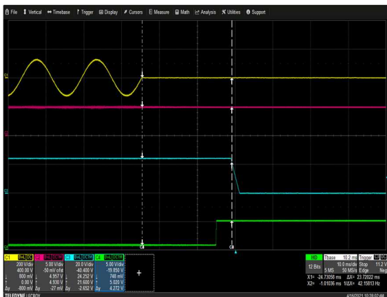
Figure 32: μMP16C-SKQ-SKQ-30-A Hold-up Time V_{in} = 90V_{ac}/63Hz Load: I_o = 41.66 I_{SB} = 2A Ch 1: AC Mains Ch 2: V_{SB} Ch 3: V_o Ch 4: Global DCOK
