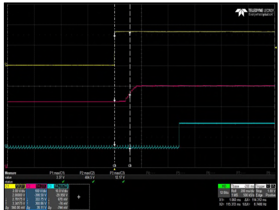
Figure 4: AIF06ZPFC-01L Turn-on delay via PF ENABLE Vin = 230Vac Load: Io = 0A Co = 2000uF Ch 1: PF ENABLE Ch 2: Vo Ch 3: LD ENABLE
